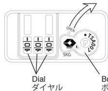
Turn the button clockwise to open the lock
